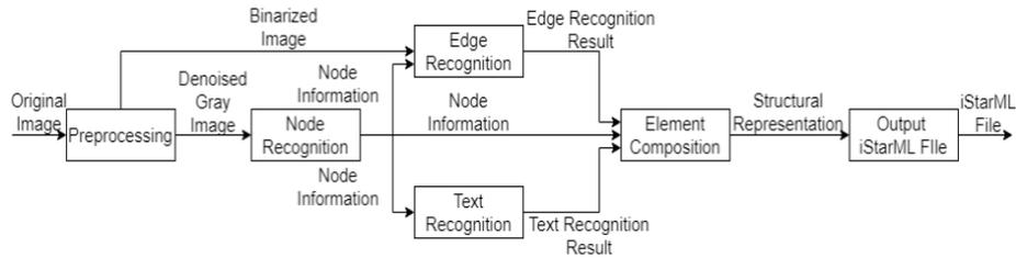
Fig. 1. Modules and Data Flows within the Proposed Framework
