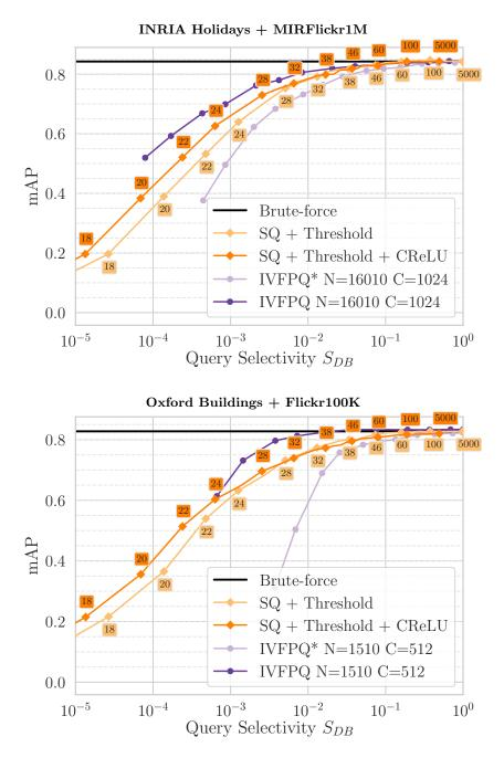
Fig. 1. Effectiveness (mAP) vs efficiency ( $S_{DB}$  — fraction of dataset accessed) tradeoffs of Scalar Quantization based (SQ) and Product Quantization based (IVFPQ) methods. Curves are produced varying  $\gamma$  for SQ (reported near each point) and the number of accessed lists (nprobe) for IVFPQ. Brute-force represents the sequential scan baseline. IVFPQ\* represents IVFPQ trained on out-of-distribution images.
