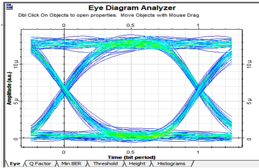
**Fig 4.3:** Outflow eye diagram at 1550 nm with 5dB amplifier.
