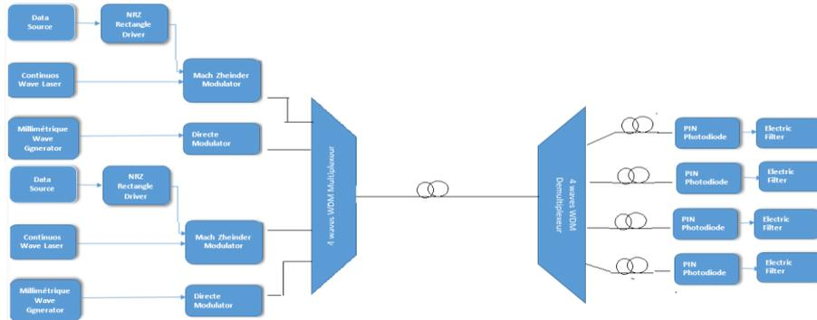
Fig 3: WDM 4 waves block diagram
