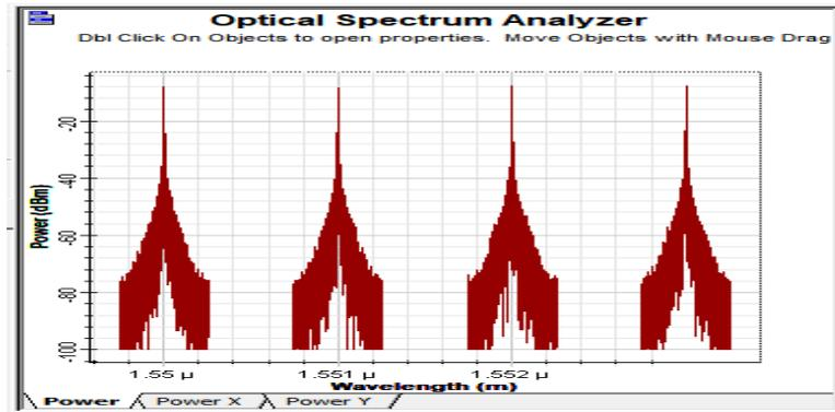
**Fig 4.1:** Spectral representation of 4 channels WDM Mux out put
