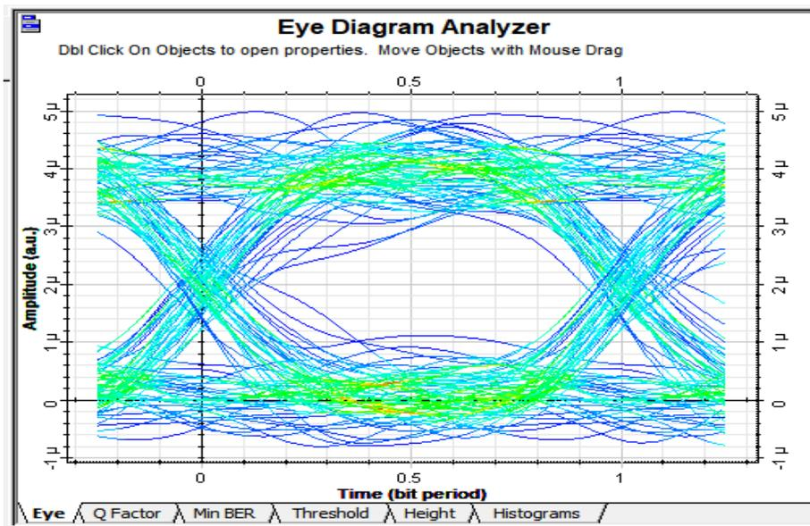
**Fig 4.2:** Outflow eye diagram at 1550 nm
