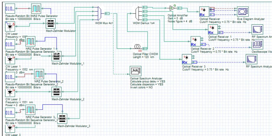
Fig 4: Four channels WDM Multiplexing
