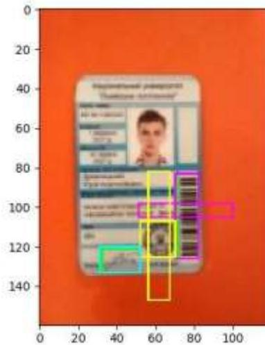
**Fig. 8.** Image for example of calculation of YOLO error green is indicated by true bbox, others include different classes
