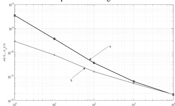
Fig. 4. The Allan deviation: (a) – previously used QFS construction, (b) – developed QFS construction.
