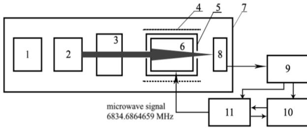
Fig. 1. The structural diagram of the rubidium QFS: 1 - reflector; 2 - a lamp with vapors of rubidium - 87; 3 - cell - filter; 4 - solenoid C - fields; 5 - radio frequency resonator; 6 - a cell with buffer gas; 8 - photodetector; 9 - automatic frequency control system; 10 - highly stable crystal oscillator; 11 - frequency synthesizer.
