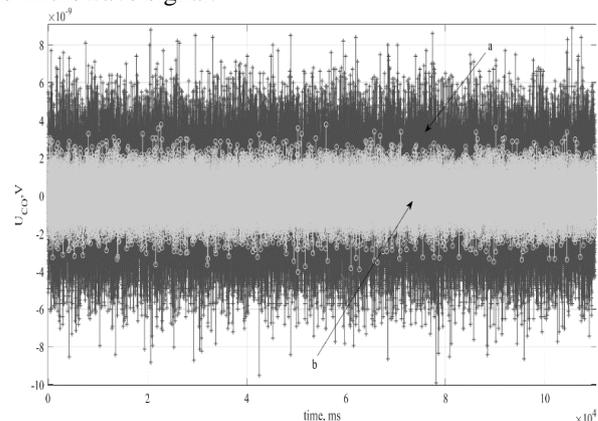
Fig. 2. The phase noise amplitude of error signal. (a) – corresponds to the earlier value of the error signal with simple accumulation, (b) – error signal using median filtration.
