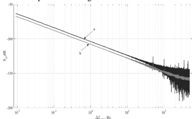
Fig. 3. The phase noise spectral power density of error signal: a - the previous version of the software; b - the new version.
