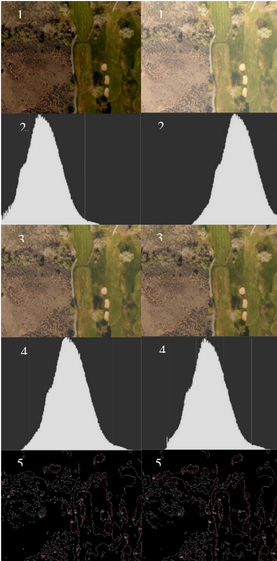
Fig. 7. Process of image brightness normalization and matching, from the two source image with different luminosity, to the results, BIM's shape detection.
