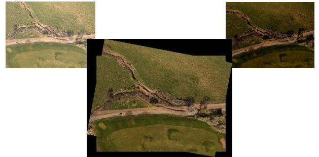
Fig. 1. Illustration of the objective of brightness normalization: Matching two images with different exposition.
