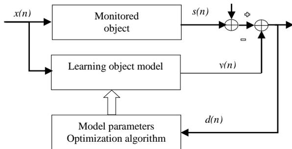
Fig. 6. Block diagram of adaptive parametric identification.
