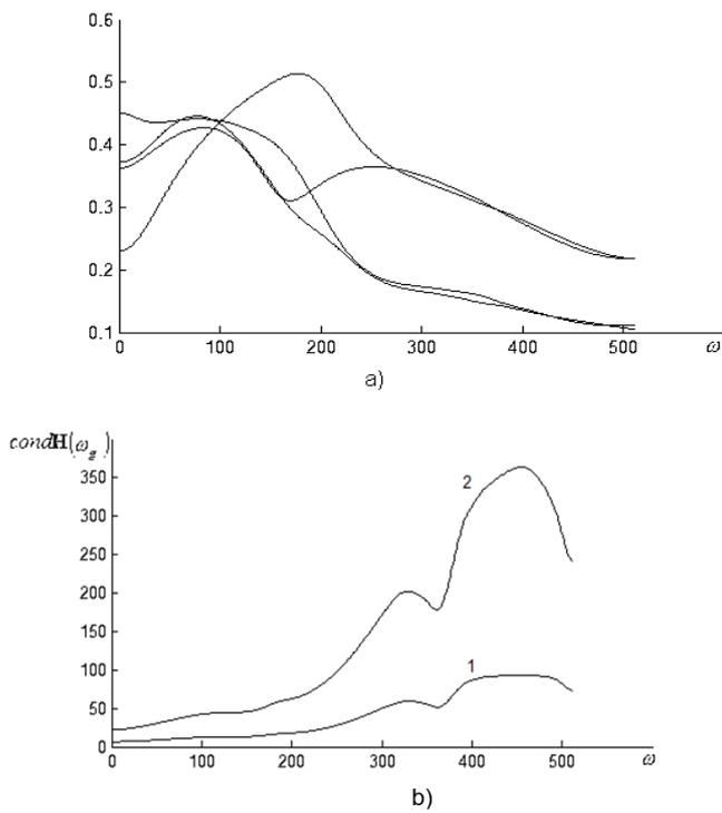
Fig. 3. a) Frequency response of the channels of matrix  $\mathbf{H}(\omega_g, 1)$ ; b) the relationship between the condition number  $cond\mathbf{H}(\omega_g, 1)$  of the mixing matrix and the frequency.
