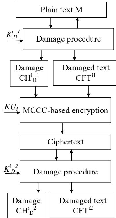
Fig. 1. Block diagram of a hybrid crypto-structure construction based on the ciphertext damage.
