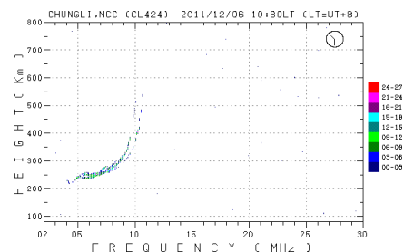
Fig. 1: An example of an ionogram. Color indicates the intensity of reflection. This is the form in which an ionosonde initially receives the data; all other parameters are determined from this image.
