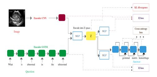
Fig. 3. Overview of the proposed VQA system based on variational autoencoders for radiology images. Input questions are encoded by an LSTM. Images are encoded by a CNN.
