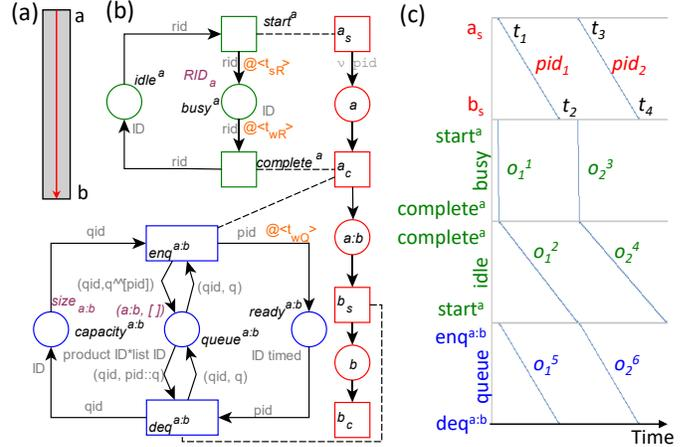
Fig. 1. The MHS conveyor (a), corresponding PQR-system (b) and PS (c).
