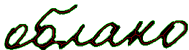
Fig. 1. Contour representation (green line) and skeleton (red line) of a binary image.
