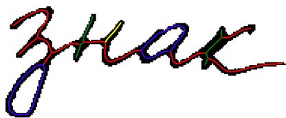
Fig. 3. Skeleton graph decomposition into strokes: cyclical (blue), vertical (green), semi-vertical (yellow) and simple (red).
