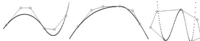
Fig. 2. Construction of the smooth cubic spline by 4 points.
