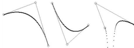
Fig. 3. Construction of the Bezier curve by means of local-geometric approach
