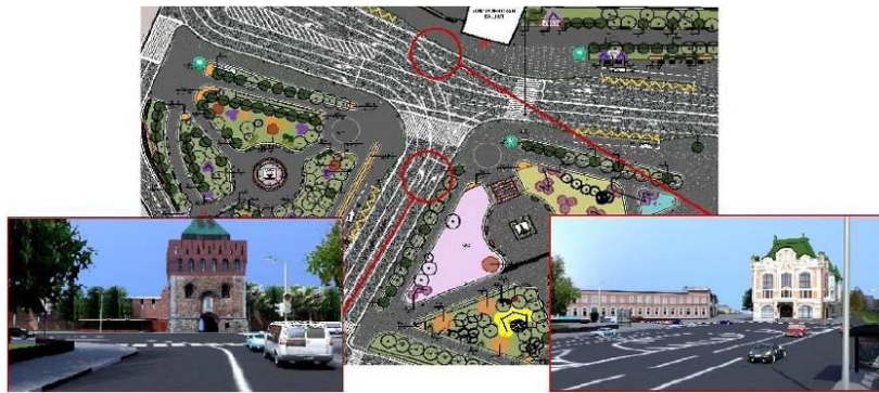
Fig. 2. Images of low-polygonal three-dimensional scenes (bottom), which are examples of Object for recognizing via the Vuforia Object Scanner one of the city square from the positions marked by tags on the map (top).
