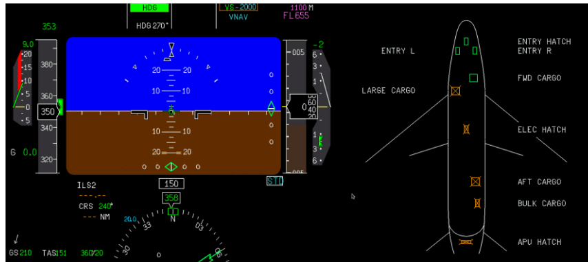
Fig. 2. Multi-window visualization of two applications – PFD and DOORS.
