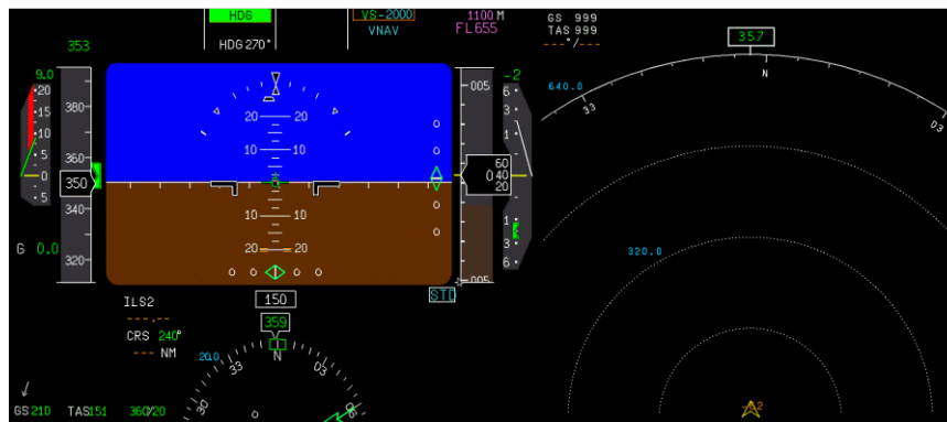
Fig. 3. Multi-window visualization of two applications – PFD and ND.
