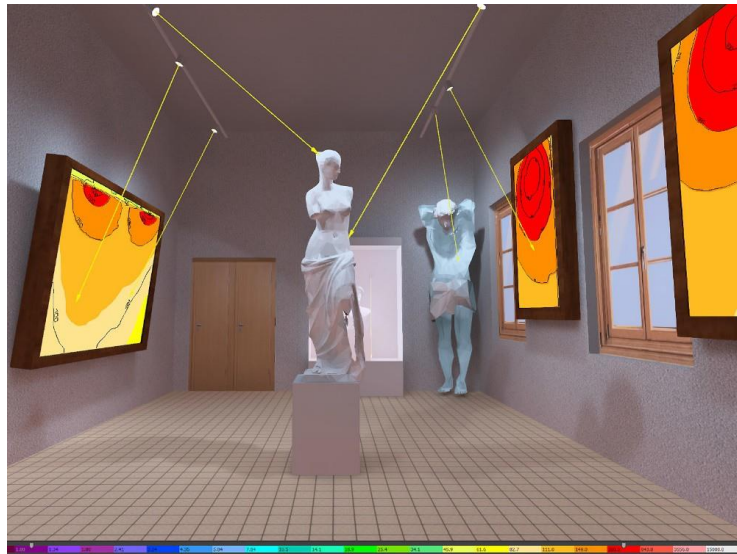
Fig. 2. The engineering approach in lighting (MPEI). Searchlights are arranged according to the task. The targeting of lighting devices and the light levels on the exhibits are shown.
