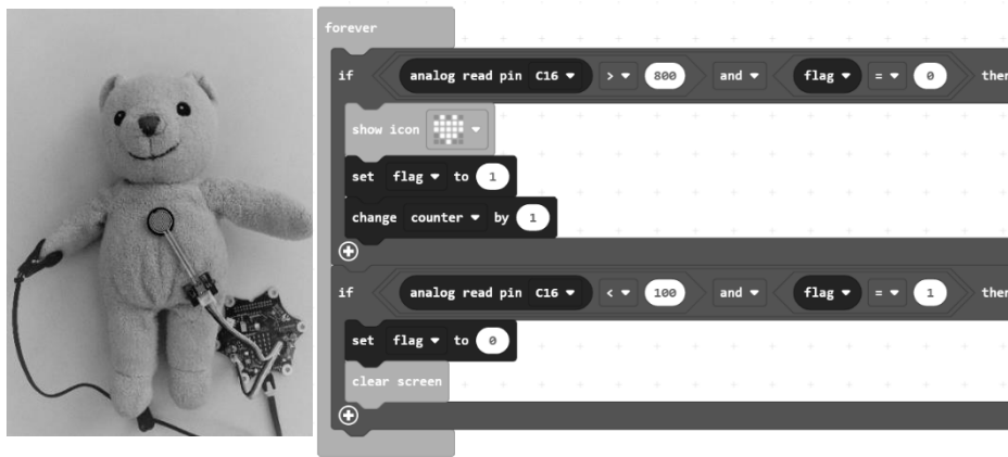
Fig. 4. computer system for a resuscitation phantom
