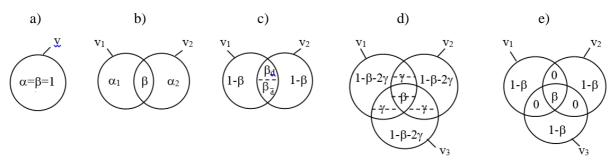
Figure 5: Models of faults sets of one-version (a), two-version (b,c) and three-version (d,e) CPS
