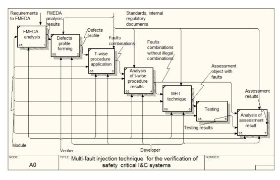
Figure 4: IDEF diagram of multi-FIT technique [12]
