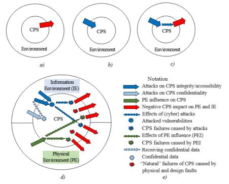
**Figure 1:** Models of CPS safety and security: model of safety (a), models of security (b) and influence of security on safety, model of interaction of CPS and environment (d), notation of models
