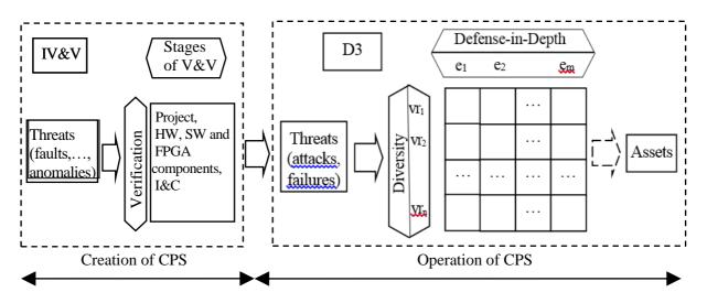
**Figure 3:** Two echelons of CCF protection: independent verification and validation and D3 (defencein-depths and diversity) approach: ei–echelons of protection in depth, vr– types of version redundancy
