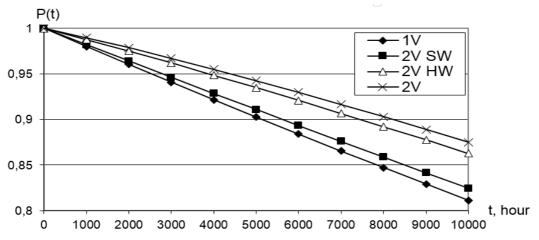
**Figure 6:** Dependencies of CPS probability of up-state on time for one-version system (1V), two-version system with diverse SW (2V SW), HW (2V HW) and as SW and HW (2V) versions
