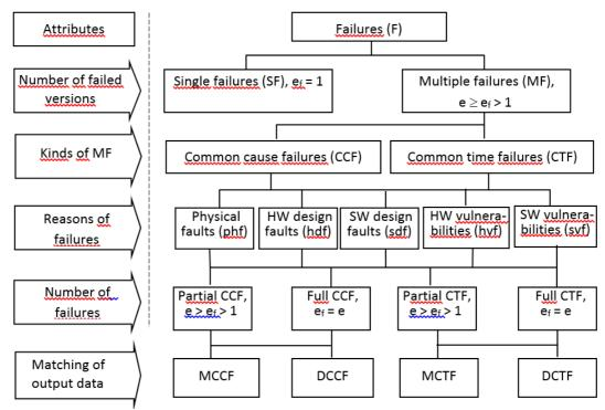
Figure 2: Classification of common cause and common time failures types and its reasons
