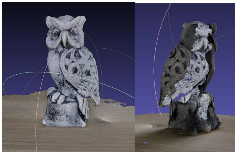
**Fig. 10.** MVS model - Screened Poisson Surface Reconstruction
