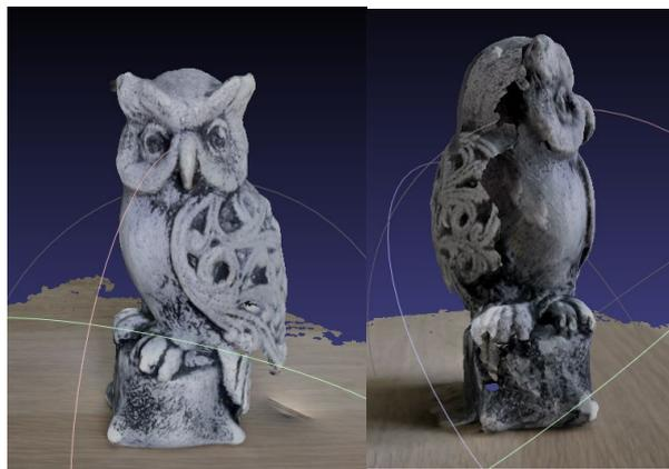
**Fig. 9.** MVS model - Floating Scale Surface Reconstruction
