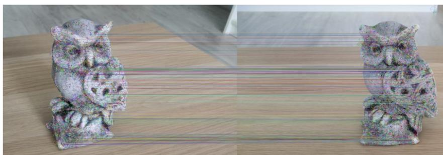
Fig. 4. The result of key point comparison for a pair of original images
