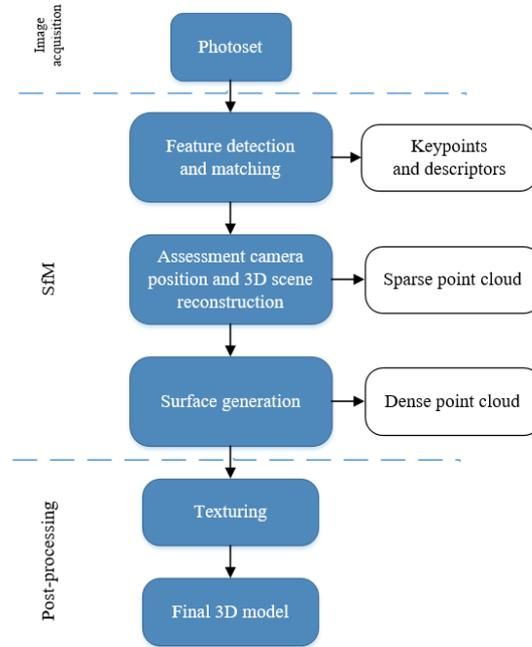
Fig. 1. Simplified process of obtaining a 3D model based on a set of images
