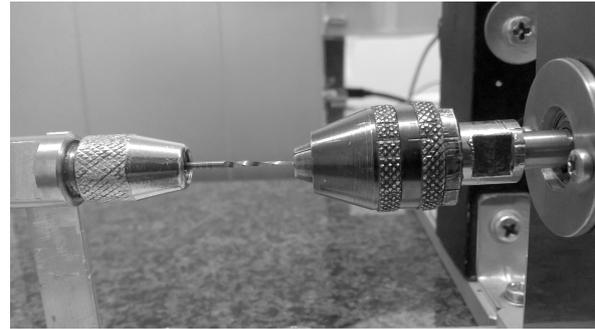
**Figure 3:** Detail of the torsion testing device.
