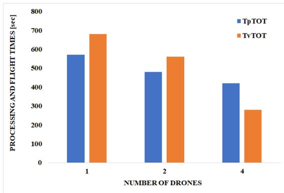
Figure 4: Flight and processing time as the number of drones varies for a  $9 \times 9$  matrix
