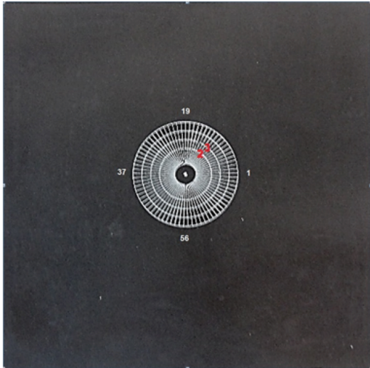
Figure 1: Left: Side for epipolar reconstruction. In white and in red meridians and parallels considered in CNN, respectively. Right: Side for DIC reconstruction. In this sample, holes for clamping are already made.
