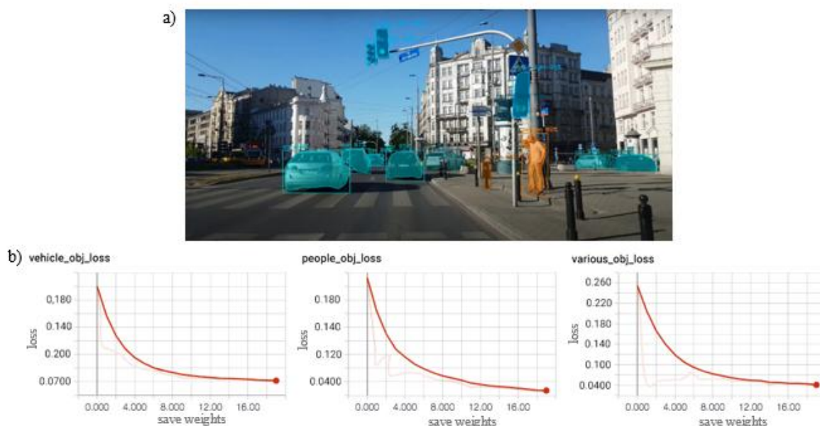
Figure 2: Results of testing the module “Collection and primary analysis of data” in traffic conditions (a – identifying objects in the incoming video stream; b – plots (wide red line – reference plot of losses; red line – plot of logged losses) of identified objects to log losses and save weights at the end of every epoch)
