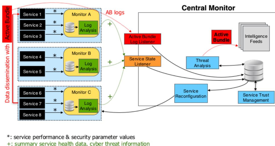
Figure 1: Solution architecture
