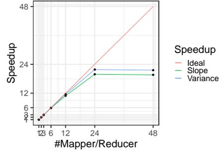
**Fig. 4.** Corresponding speedup of SEPP on 27M, using the simple linear regression model (Slope) and variance model (Variance).
