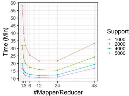
**Fig. 5.** Runtime of SEPP on the MSNBC dataset with different minimum support thresholds, in relation to different numbers of mapper/reducers.
