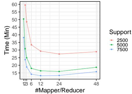
**Fig. 6.** Runtime of SEPP on the Kosarak dataset with different minimum support thresholds, in relation to different numbers of mapper/reducers.
