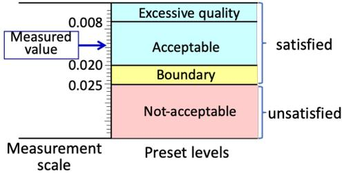
Figure 4 Typical preset rating levels
