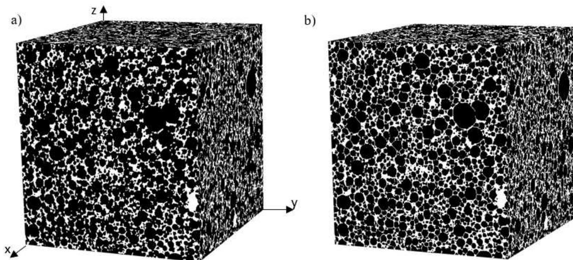
**Fig. 1.** a) Binarized 3D image before segmentation and b) after segmentation
