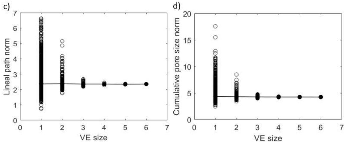
**Fig. 7.** Scatter of a) porosity; norm of b) two-point correlation function; c) lineal path function and d) cumulative pore size distribution function for each VE size along with their average values
