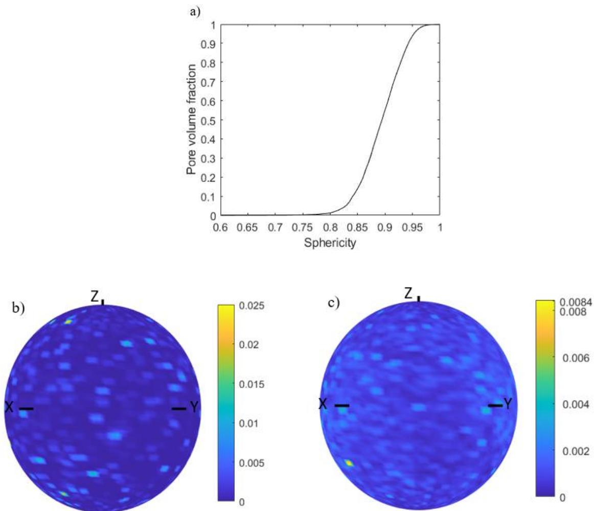
**Fig. 2.** a) Cumulative distribution of pore sphericity, b) orientation distribution of pores having sphericity  $0.75 < \psi < 0.85$  and c) orientation distribution of pores having sphericity  $0.85 < \psi < 0.95$
