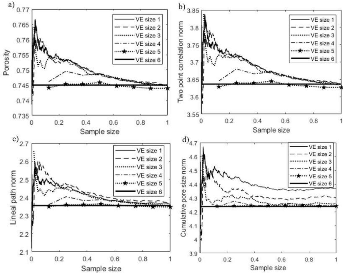
**Fig. 6.** Effect of sample size on a) porosity; norm of b) two-point correlation function; c) lineal path function and d) cumulative pore size distribution function for each VE size
