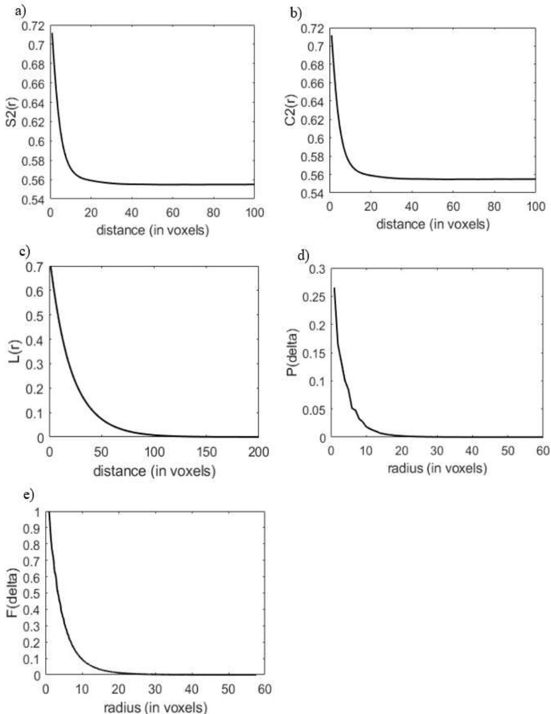
**Fig. 3.** a) Two-point correlation function; b) Two-point cluster correlation function; c) Lineal path function; d) Pore size distribution function; e) Cumulative pore size distribution function of the alumina foam sample.
