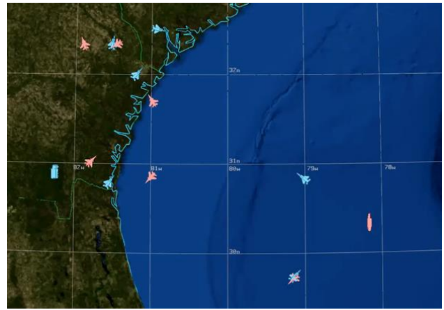
Figure 11 - Multi-agent AFSIM-based environment with 6 blue fighters and 6 red fighters. The blue station on the left and red ship on the right serve only to command their fighters. The fighters fire missiles at one another, and enemy destruction is determined based on missile dynamics and weapon models.
