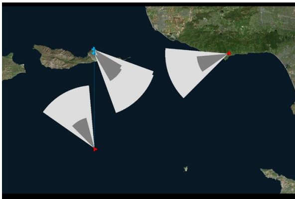
Figure 3 - Simplified MA2D environment, written entirely in Python. This example contains two blue fighters and two red fighters. Dark gray areas represent each unit's weapon zone. The objective is to destroy all opponents by getting each within this zone, while avoiding similar destruction of friendly aircraft. This simplification eliminates the need for modeling missile flight.
