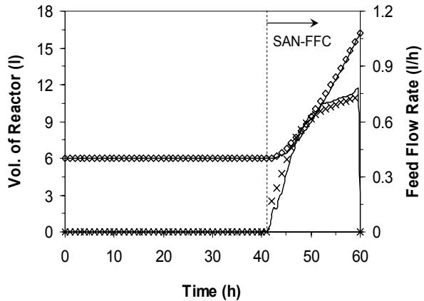
**Figure 10:** Control action of SAN-FFC in the absence of noise in *DO* measurements. The feed rate is computed from predicted values (—); the symbols represent the ideal process dynamics (× Substrate feed flow rate and ◇ volume of reactor).
