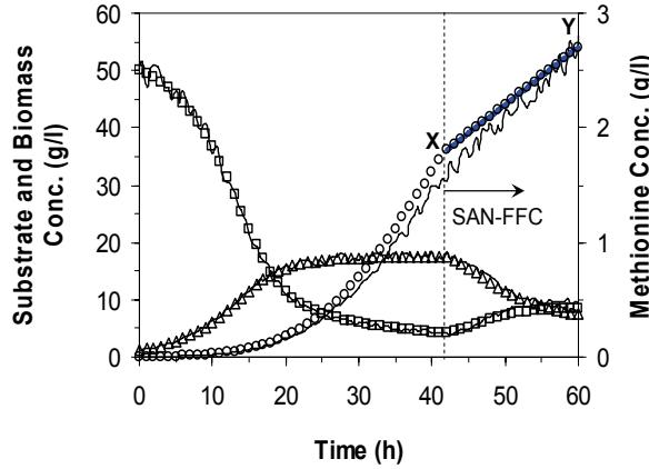
**Figure 11:** Performance of SAN-FFC strategy implementation when there is 5% noise in the DO measurements. XY shows the desired trajectory. SAN-FFC forces the process is made to converge to the desired trajectory. (—); the symbols represent the ideal process dynamics (○ Methionine □ Substrate and △ Biomass concentrations)
