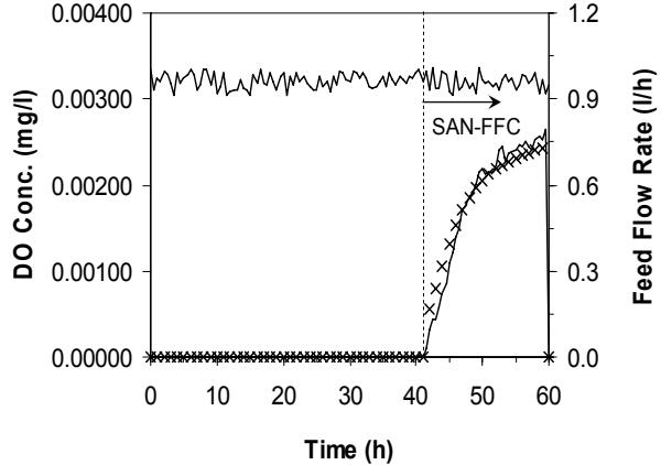
**Figure 12:** Control action of SAN-FFC when there is 5% noise in DO measurements. The feed rate is computed from predicted values (—); the symbols represent the ideal process dynamics (× Substrate feed flow rate and ◇ volume of reactor)
