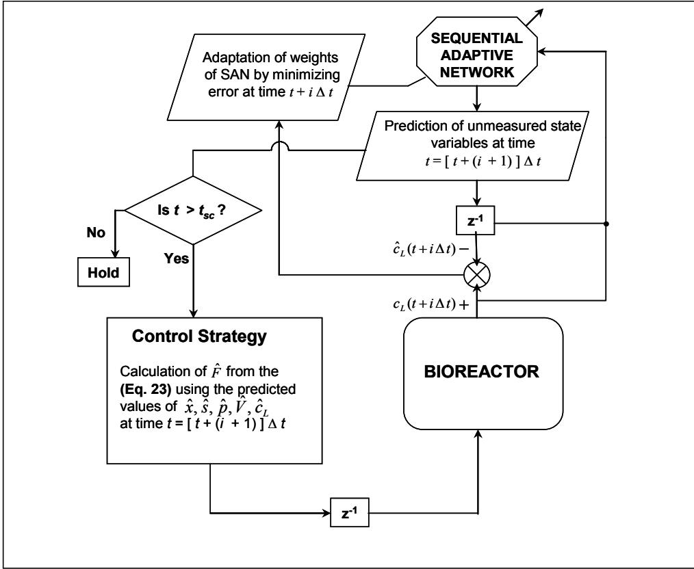
**Figure 3:** Flow diagram of SAN based feed forward control strategy for methionine production system
