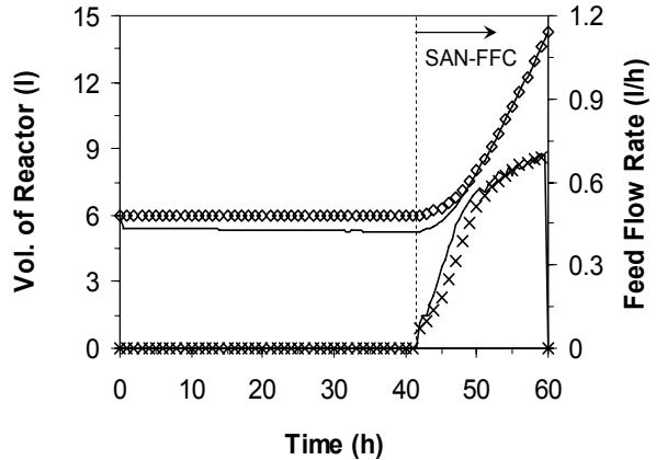
**Figure 16:** Control action of SAN-FFC when the specific growth rate  $\mu$  is varied randomly; there is no noise in DO measurement. The feed rate is computed from predicted values (—); the symbols represent the ideal process dynamics (× Substrate feed flow rate and ◇ volume of reactor).
