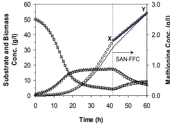
**Figure 9:** Performance of SAN-FFC strategy implementation in the absence of noise in the *DO* measurements. XY shows the desired trajectory. SAN-FFC forces the process is made to converge to the desired trajectory. (—); the symbols represent the ideal process dynamics (○ Methionine □ Substrate and Δ Biomass concentrations).
