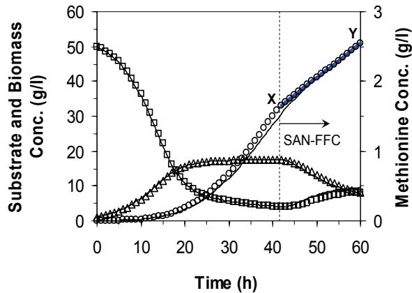
**Figure 15:** Performance of SAN-FFC strategy implementation when the specific growth rate  $\mu$  is varied randomly; there is no noise in DO measurement. XY shows the desired trajectory. SAN-FFC converges quickly to the desired trajectory. (—); the symbols represent the ideal process dynamics (○ Methionine □ Substrate and Δ Biomass concentrations).
