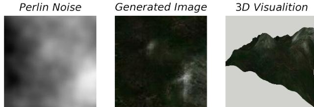
**Figure 10: The well known technique of generating DEMs with random Perlin noise, is enhanced by adding plausible colors to the random DEM, using the trained inverse CGAN model.**
