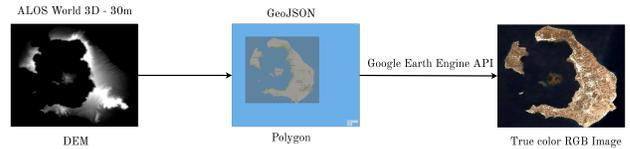
Figure 3: Flow chart of the satellite-imagery dataset collection process using the Google Earth Engine API. The outermost points of the georeferenced DEM are selected as the boundary for the GeoJSON Polygon, which when fed into the API returns the corresponding RGB satellite image.
