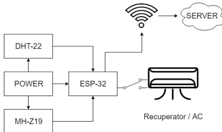
Fig. 4. Scheme of the microclimatic module
