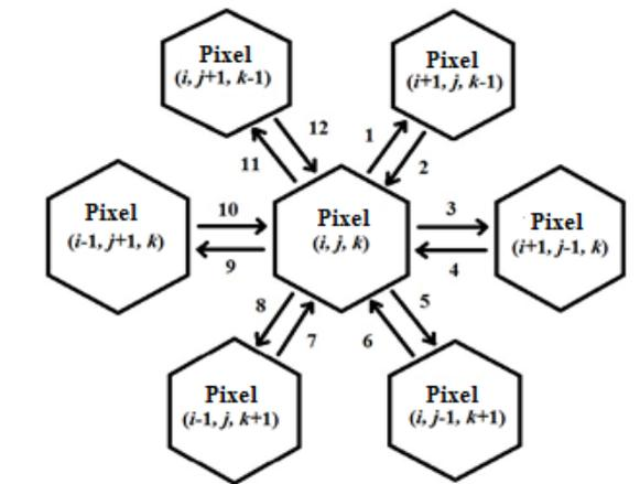
**Fig. 2.** Hexagonal lattice, which binds six neighboring pixels in the model of the biopixels using the cubic coordinates:
