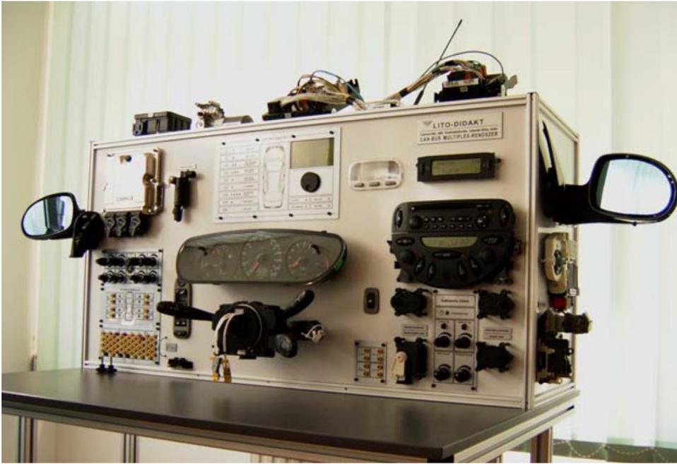
**Figure 8.** The Citroen C5 test bench.
