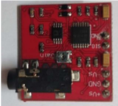
Figure 3: Myoware EMG Sensor
