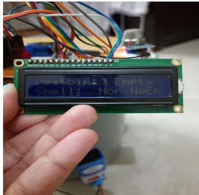
Figure 4: LCD displays the message according to the smell detected and the pan's then status of fullness
