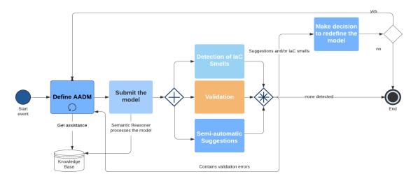
Figure 2: BPMN model describing the AADM authoring workflow.
