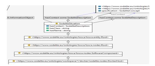
Figure 4: sodalite.nodes.DockerHost custom node type as a UML graph in Topbraid ME Composer
