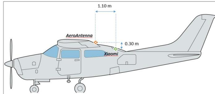
**Figure 2:** Leverarm between smartphone antenna and the AeroAntenna
