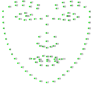
Figure 3: The facial key points generated by OpenFace [23]
