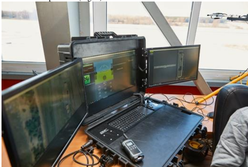
Fig. 3. The center for information control of the SKYF work
