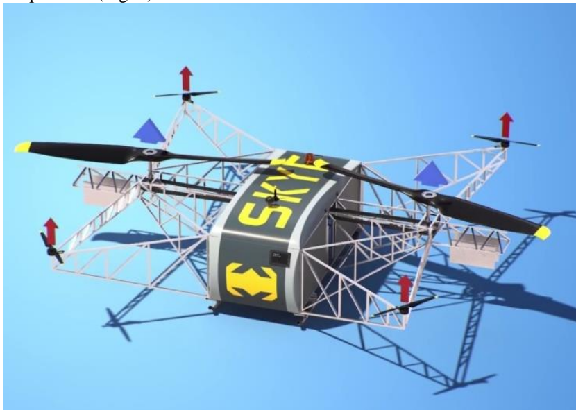
Fig. 2. The schematic diagram of the action of the lifting and tail screws
