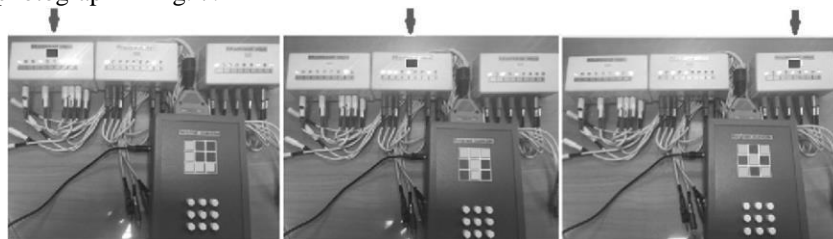
Fig. 7. Appearance of a perceptron based on selective neurons configured to recognize the letters of the English alphabet L, T, X. An experiment on the recognition of letters L, T, X is shown
