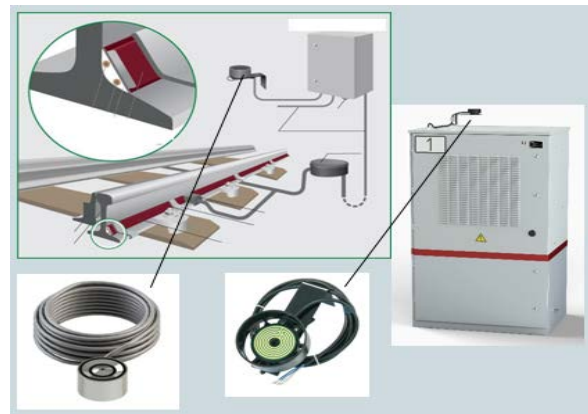
Figure 4: Principle of operation and installation diagram for electro-thermal ice/snow buildup sensor
