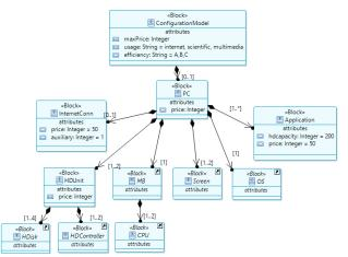
Figure 6. Product architecture of the configuration model.
