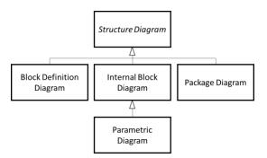
Figure 1. Excerpt of SysML diagram taxonomy [4]
