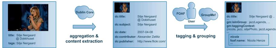
Fig. 4. Example: process of RDF content creation
