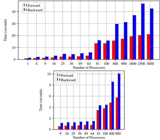
Figure 5: Weak scaling runtime for forward computation and gradient back-propagation. Top: each MPI processor has 1 core; bottom: each MPI processor has 4 cores. We see a jump near 64 cores because this is where network communications start to take place (recall each of our CPUs has 32 cores, and each node has two CPUs). The plots show results of weak scaling, each MPI processor solves a local problem of the same size.
