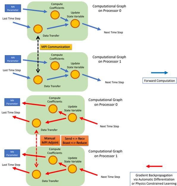
Figure 1: Paradigm for distributed machine learning for computational engineering. The data communication operations are treated as nodes in the computational graph. They are separate from the other computing operators. This makes it easy to reuse existing serial implementations of the numerical PDE solver.
