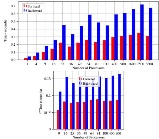
Figure 6: Overhead of ADCME for matrix solving in Hypr. The top and bottom bar plots correspond to the top and bottom ones in Fig. 5.
