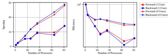
Figure 8: Speedup and efficiency for parallel computing of the Poisson's equation.
