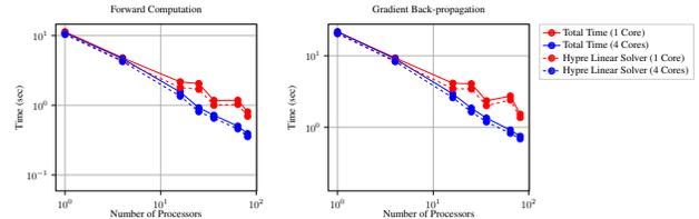
Figure 7: Runtime for forward computation and gradient back-propagation. The plots show results of strong scaling, the whole problem size is fixed and we increase the number of MPI processors (each processor has 1 or 4 cores).
