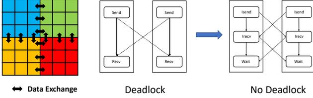
Figure 2: Left: domain decomposition and halo exchange pattern. Two adjacent patches exchange boundary information. Right: using nonblocking sends/receives to avoid deadlocks.
