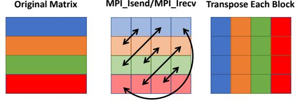
Figure 3: Transposition of a distributed sparse matrix. Each block exchanges nonzero entries with the corresponding transposed block. The original and resulting matrices are both stored in CSR formats.
