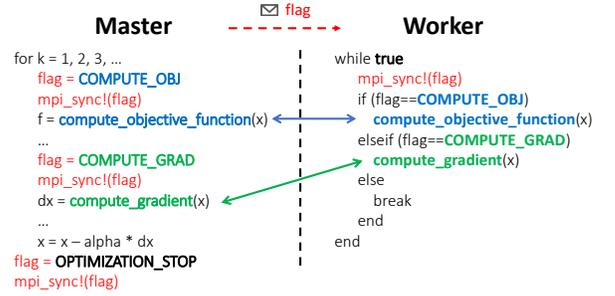
Figure 4: Refactoring a serial optimizer to an MPI-based optimizer in our framework.
