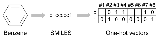
Figure 3: Example of SMILES representation and one-hot vectors for benzene. For simplicity, only two characters are shown in the one-hot encoding. In practice, one-hot vectors forms M \times N matrix, where M is the number of SMILES symbols and N is the maximum length of SMILES strings.
