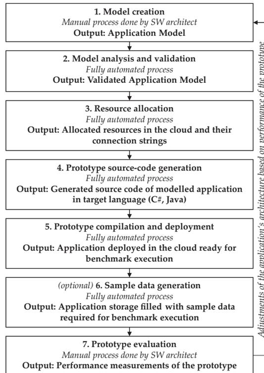
**Figure 1:** Prototyping process
