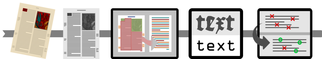
Figure 1: Main steps of a typical OCR workflow, from left to right: preprocessing, binarization, segmentation / layout analysis, recognition, and postcorrection.
