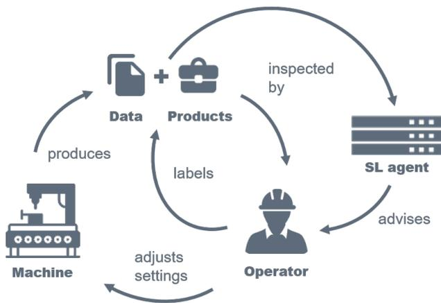
Figure 2: Assisted production using agent trained with supervised learning (SL) during operation.
