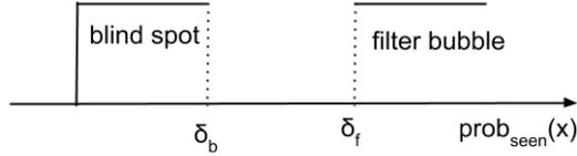
**Figure 6:** The blind spot and filter bubble in a recommender system. Here,  $\delta_b$  represents the threshold up to which items that have a lower probability of being seen will not be discovered by users. On the other hand, items with probability of being seen higher than  $\delta_f$  will likely be discovered by users.
