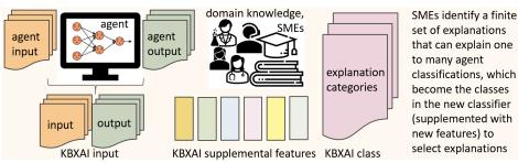
Fig. 1: Overview of KBXAI: Step 1 obtains explanation categories; Step 2 supplements the data with new features to select explanations to explain classifications
